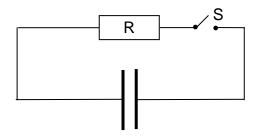
Which ONE of the following correctly describes the changes in the current, *I*, in the circuit and the potential difference, *V*, across the capacitor when the switch S is closed?
