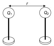
The distance between the charges is now **halved** and the charge on  $Q_1$  is **doubled.** The magnitude of the new force between the charges is ...
