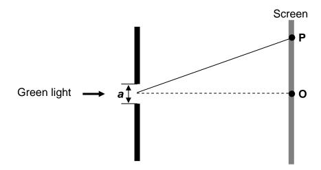
Which ONE of the following changes regarding the colour of the incident light and the width of the slit will cause the GREATEST increase in the distance OP?
