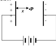
The magnitude of the electric field at **P** is *E*. At a distance  $\frac{1}{2}x$  from the positive plate, the magnitude of the electric field will be ...
